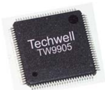
Techwell's TW9905 100-pin LQFP package
